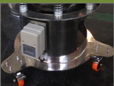
SOLID STRONG BASE WITH WHEELS FOR PORTABILITY
