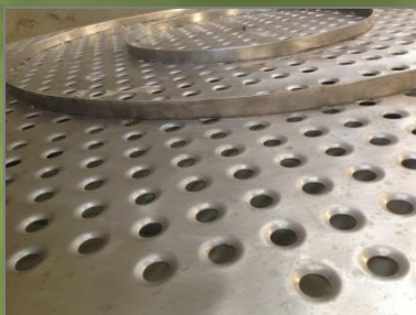
REINFORCEMENT PLATE FOR STRENGTH OF SIEVE
